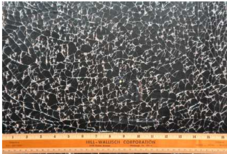
Figure 1. Breakage pattern of tempered glass.
