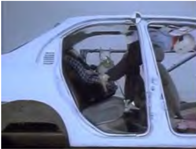
Figure 4: Capture taken from a crash test video of a frontal impact with an unbelted child crash test dummy in the rear seat. 15
