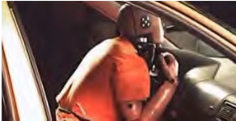
Figure 3: Unbelted crash test dummy during a 30 km/h impact.
