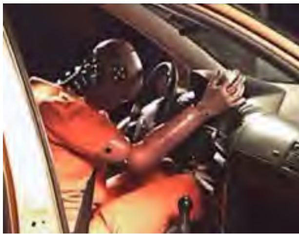
Figure 2: Belted crash test dummy during a 30 km/h impact.
